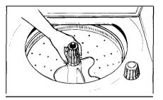
• Agitator. Remove the agitator at regular intervals—about 4 to 6 months—and remove any lint that may have accumulated. After removing the front access panel, as shown at right, unscrew the agitator cap, grasp the agitator with both hands, and pull it up and out of the washbasket.
